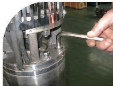
拆卸放气孔丝堵 Disassemble the gas vent plug;
